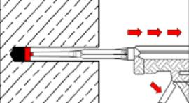
Retaining washer and mixer nozzle extensions shall be used according to Table B5 for the following applications: <ul style="list-style-type: none"><li>• Horizontal installation (horizontal direction) and ground installation (vertical downwards direction): Drill bit-Ø <math>d_0 \geq 18</math> mm and anchorage depth <math>h_{ef} &gt; 250</math>mm</li><li>• Overhead installation: Drill bit-Ø <math>d_0 \geq 18</math> mm</li></ul> |
