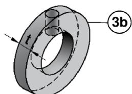
Thickness of washer with bore for diameter
