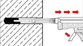
Starting from the bottom or back of the cleaned drill hole fill the hole up to approximately two-thirds with adhesive. Slowly withdraw the static mixing nozzle as the hole fills to avoid air pockets. If the drill hole ground is not reached, an appropriate extension nozzle shall be used. Observe working times given in Table B6.                                                                                                       |
