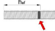
Prior to inserting the rod into the filled drill hole, the position of the embedment depth shall be marked on the threaded rod or rebar                                                                                                                                                                                                                                                                                                         |
