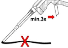
Prior to dispensing into the drill hole, squeeze out separately a minimum of three full strokes and discard non-uniformly mixed adhesive components until the mortar shows a consistent grey colour.                                                                                                                                                                                                                                            |
