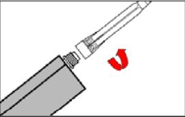
Attach the supplied static-mixing nozzle to the cartridge and load the cartridge into the correct dispensing tool.<br>For every working interruption longer than the recommended working time (Table B6) as well as for new cartridges, a new static-mixer shall be used.                                                                                                                                                                       |
