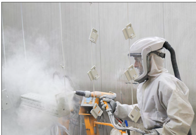
Powder coating with a spray gun
