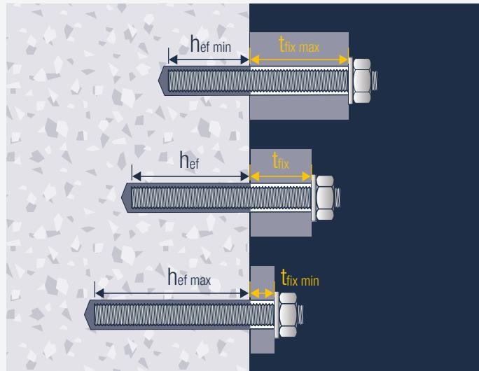
The anchor rod can be installed to a minimum anchoring depth, depending on the thickness of the attachment to be connected. The anchor rod can also be embedded deeper into the building structure, taking into account the load and clamping strength.
