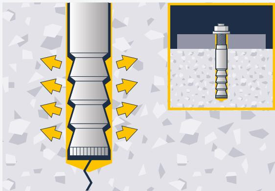
The combination of a conical anchor rod with 2-component injection resin combines the advantages of bonded and expansion anchors in a crack-resistant system.
